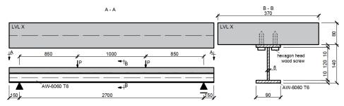
Fig. 1. The analysed aluminium and timber composite beam: A-A - top view, B-B - cross-section
