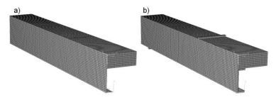
Fig. 4. Meshed composite beam: a) analysed beam b) beam with rendered shell thickness
